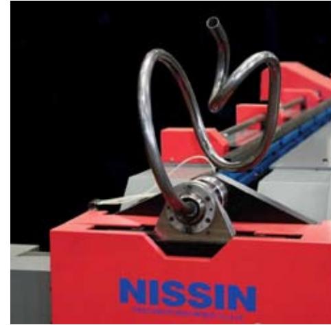
Aluminum Frame CNC Bent to Shape, stretch formed and heat treated
